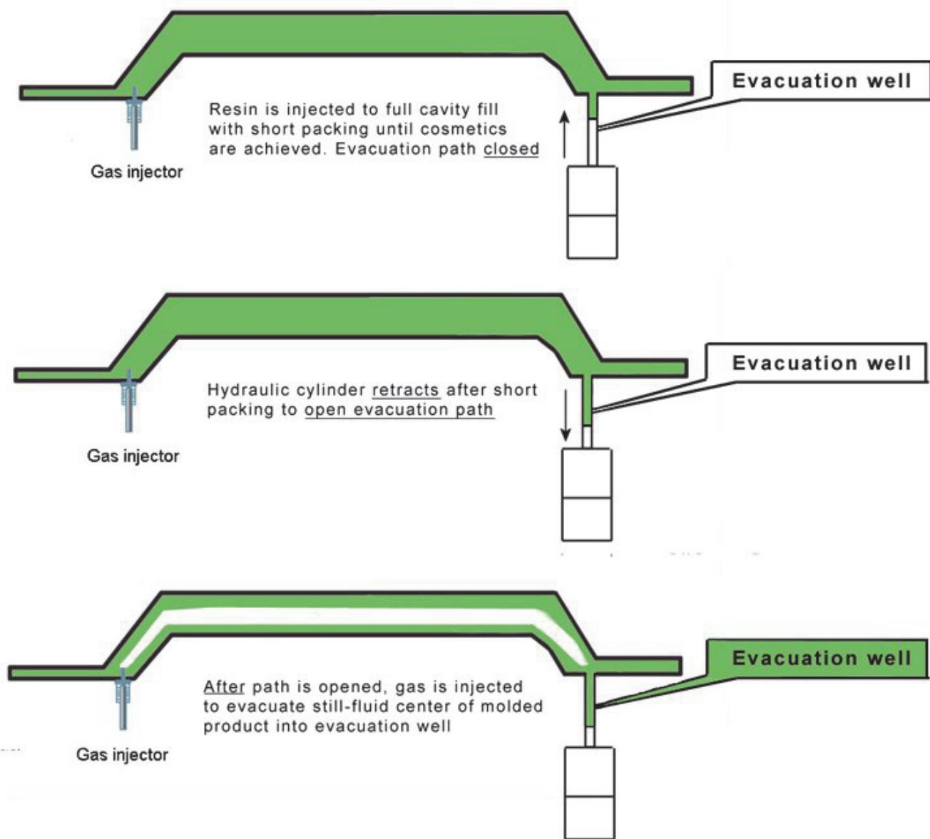
Note that in the above-described process, Class A cosmetics are achieved by using molding machine packing pressure to the resin-filled cavity prior to the gas injection phase. This hold phase timing is determined during process development – if a thicker remaining wall is desired, the hold time is increased; hold time is decreased if a thinner remaining wall is desired. The gas injection profile can also be adjusted to change the remaining wall thickness.
