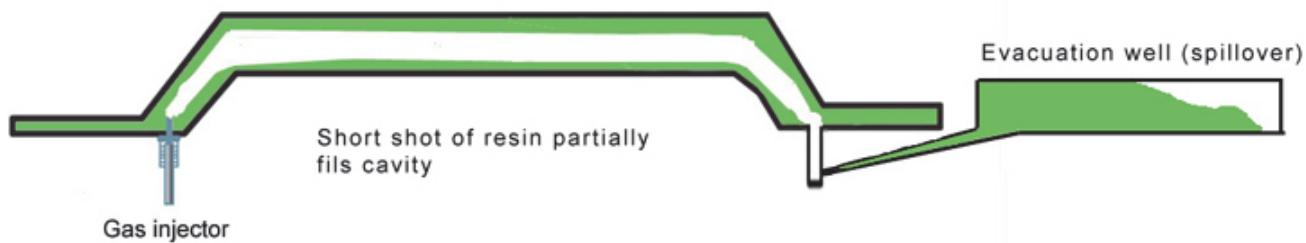
The first image above shows a cavity only partially filled with resin – short-filling was part of the patented gas assist process. Why a short shot? A short shot was necessary to prevent an uncontrollable amount of resin from exiting the flow path during the resin fill phase, or remaining in the part cavity. In the mid or late 1980's this was state-of-the-art, but has long since been replaced with far superior methods.
